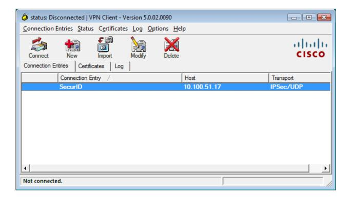
2. Click the **New** button to create an RSA SecurID connection entry. Fill in the appropriate information for the connection. The group name and password must match the entry you create on the VPN server device.
